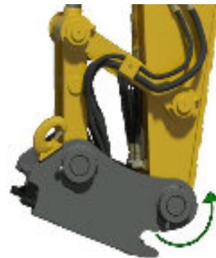
Fig 1. Positive torque direction
